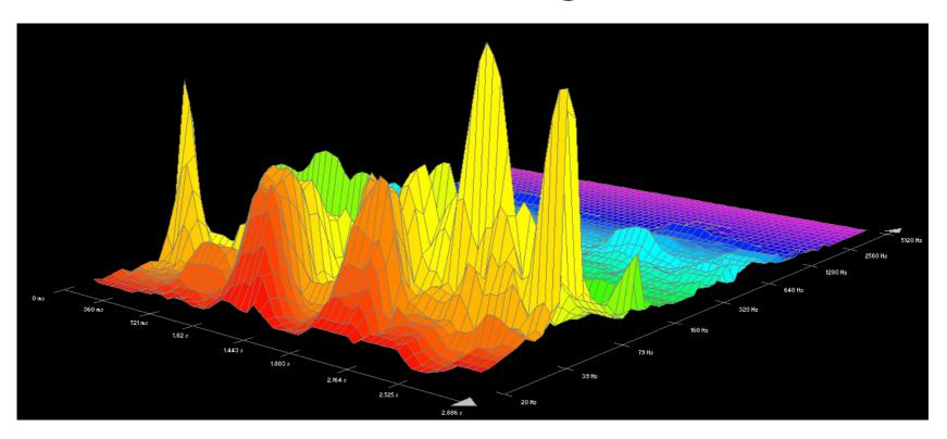
Color for indication of frequency bands ... too many degrees of freedoms in the software for visualization may lead to unintended results (here viewing angle!)
