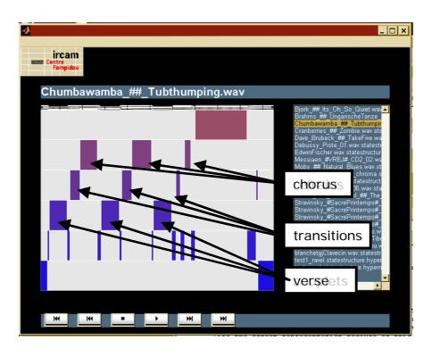
"Media Player" prototype allowing to navigate through the temporal structure of a song, similar parts are indicated by same colors and height of the boxes [Peeters, IRCAM]
